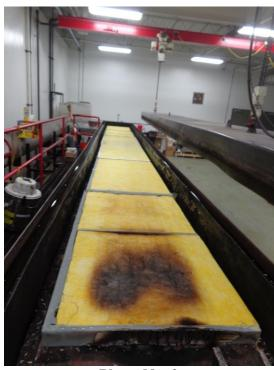
Photo No. 2 Specimen Mounted (Post-test)
